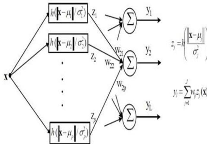
**Fig. 2** Radial Basis Function Structure.
